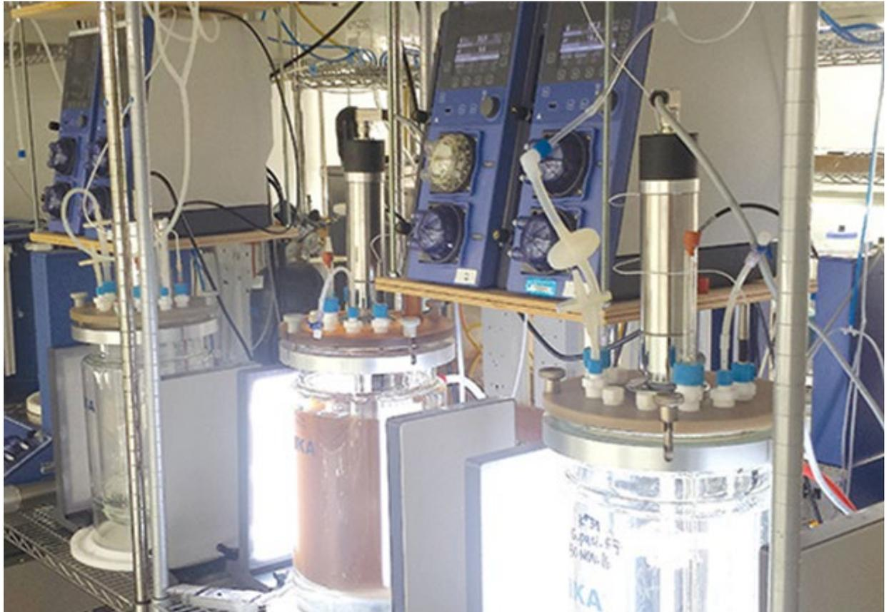
*A bioreactor, manufactured by IKA, spins in a temperature-controlled lab at UNCW's Center for Marine Science.
